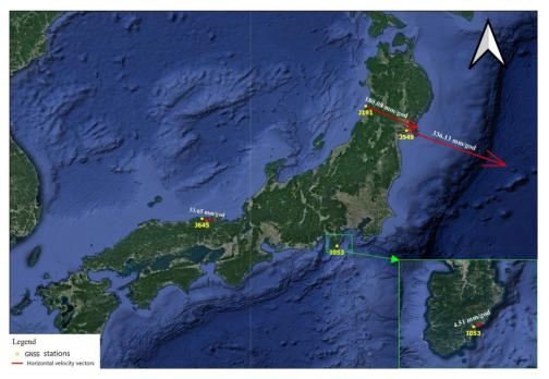
Figure 9. Horizontal velocities of GNSS stations (source: author)
