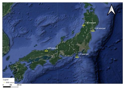
Figure 10. Vertical velocities of GNSS stations (source: author)
