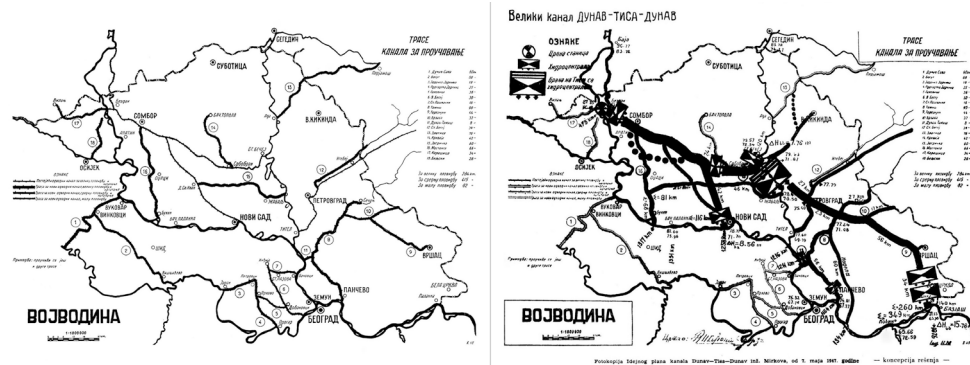
Figure 1. Left: the existing waterways in Vojvodina in 1945, with proposals for new canals in 1945-1947 (bold) [6:25]. Right: Nikola Mirkov's concept for the DTD canal network in 1947 [7:9].
