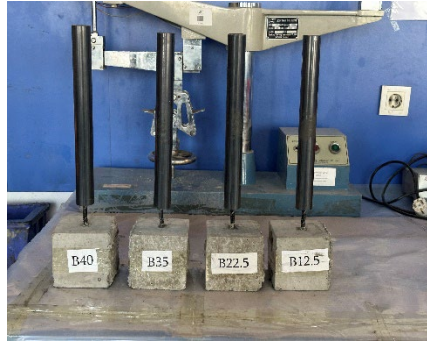
Figure 3. Test specimens. ("photography by author")
