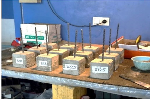
Figure 2. Concrete cubes anchored with basalt composite reinforcement. ("photography by author")
