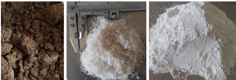
Figure 1. Materials used: (a) clay; (b) PVC waste 2/2,5mm; (c) quick lime (Photo by Feriel Berrahou)
