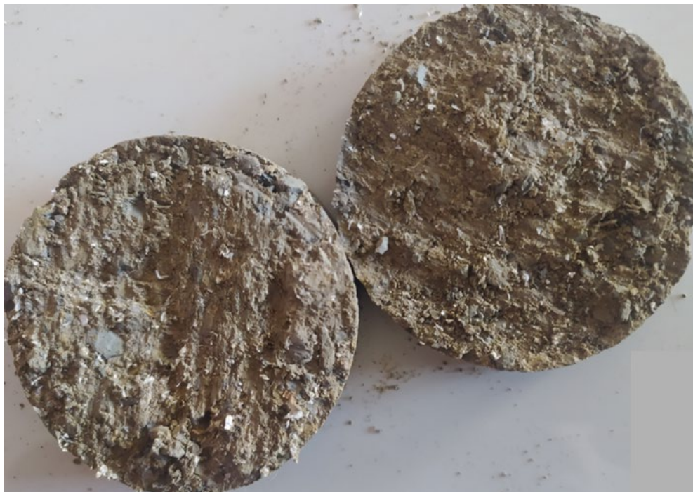
Figure 6. Specimen of treated soil after failure
