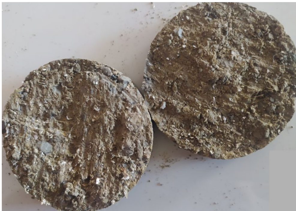
Figure 6. Specimen of treated soil after failure (photography by author)
