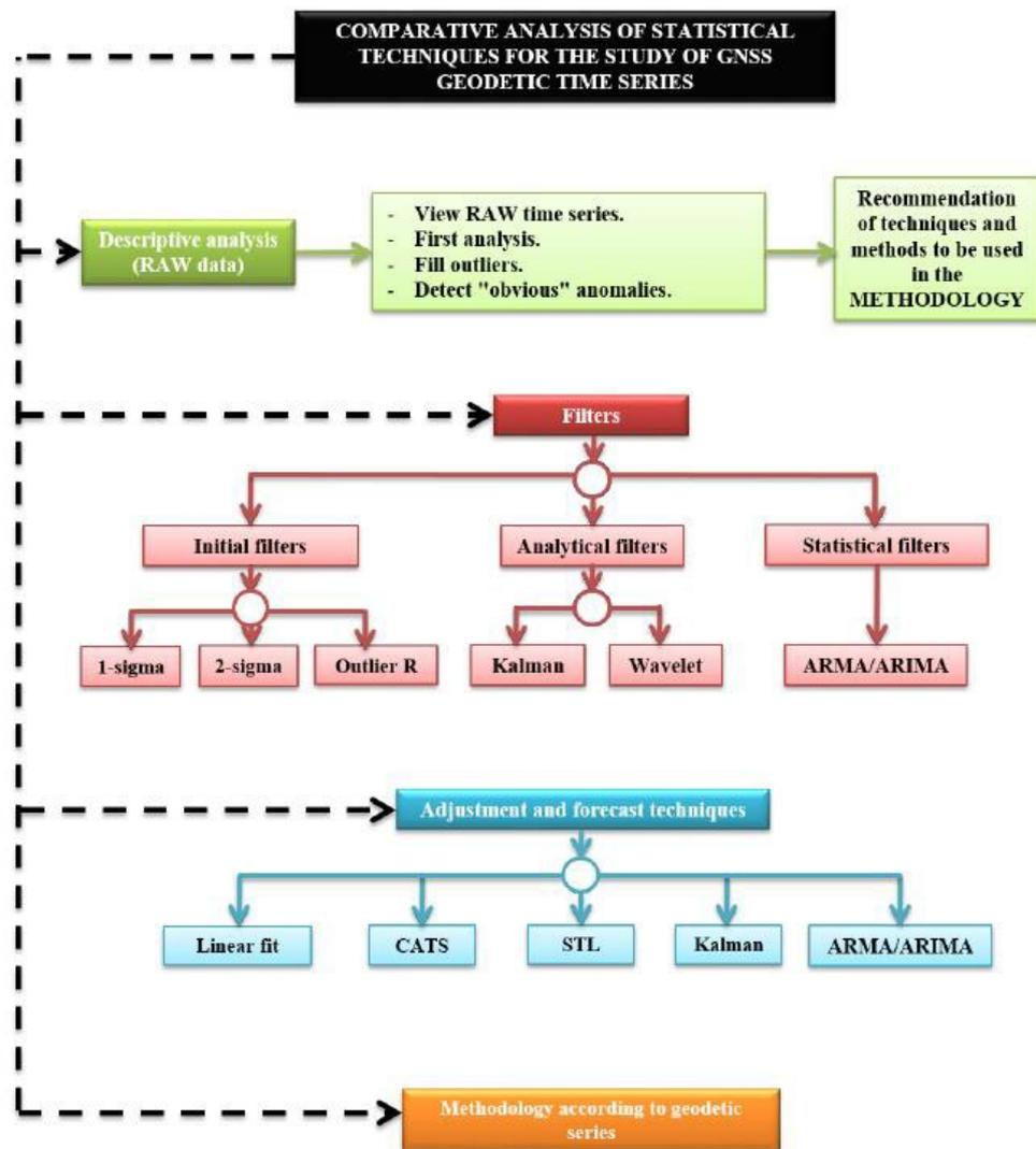
Figure 3. Methods of analysis of GNSS time series [14]
